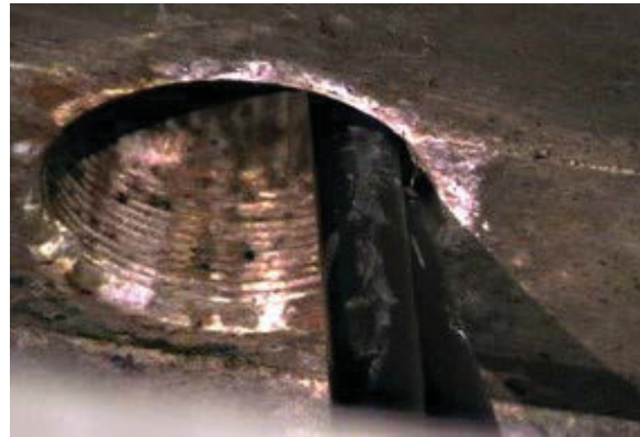
Figure 7.17. Contacting conduit edge. Photo courtesy of EPRI.
