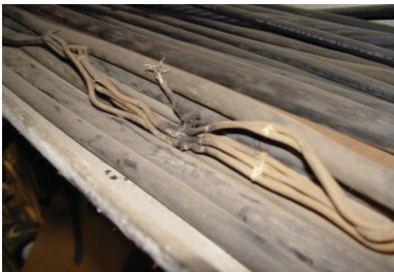
Figure 7.18. Cable short – exposed conductor. Photo courtesy of EPRI.
