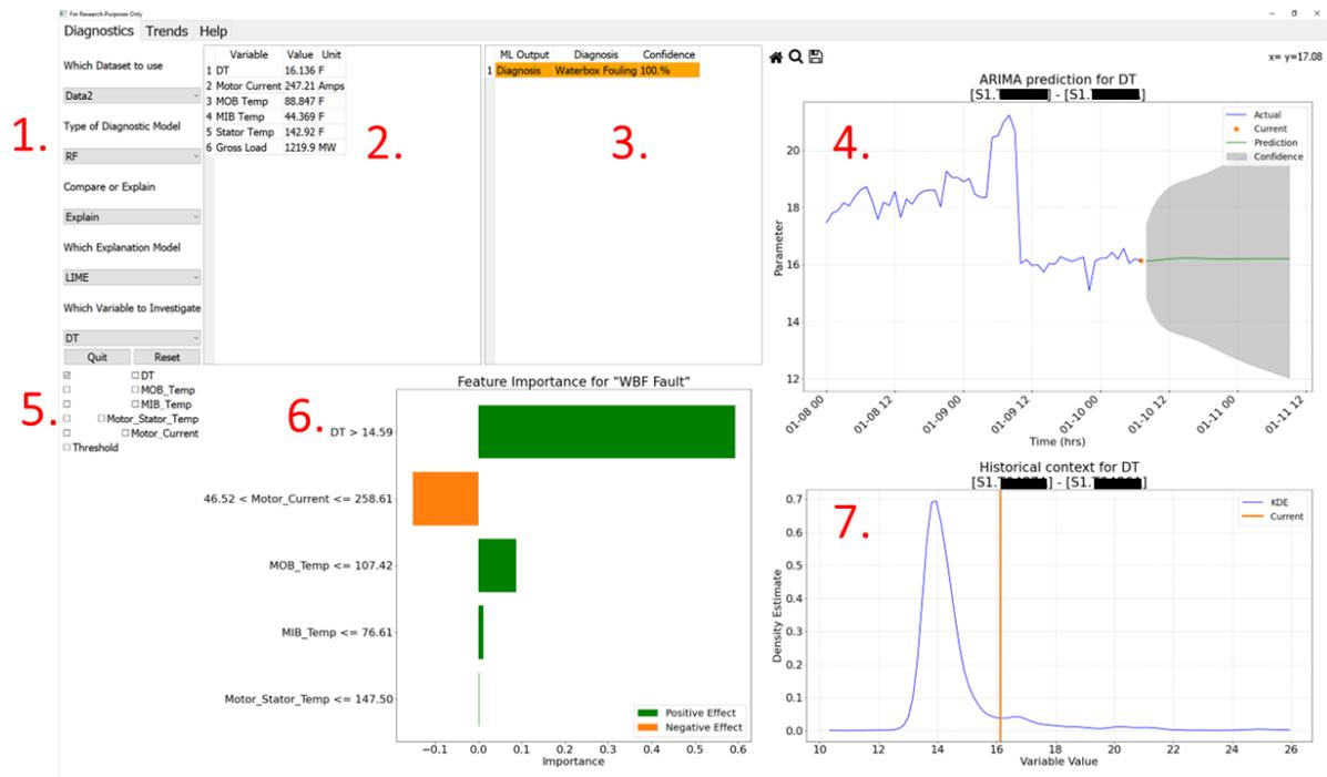
Figure 33. Front page of the M&D operator-version of the application.
