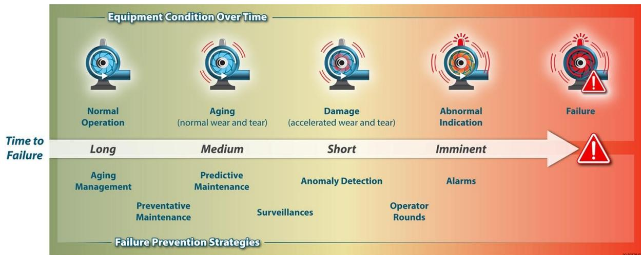
Figure 1. Equipment condition stages and strategies to prevent equipment failure.
