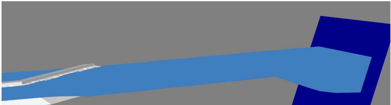
Figure 13: Ocean volume consists of 12 million particles with a flat plane used for wave generation
