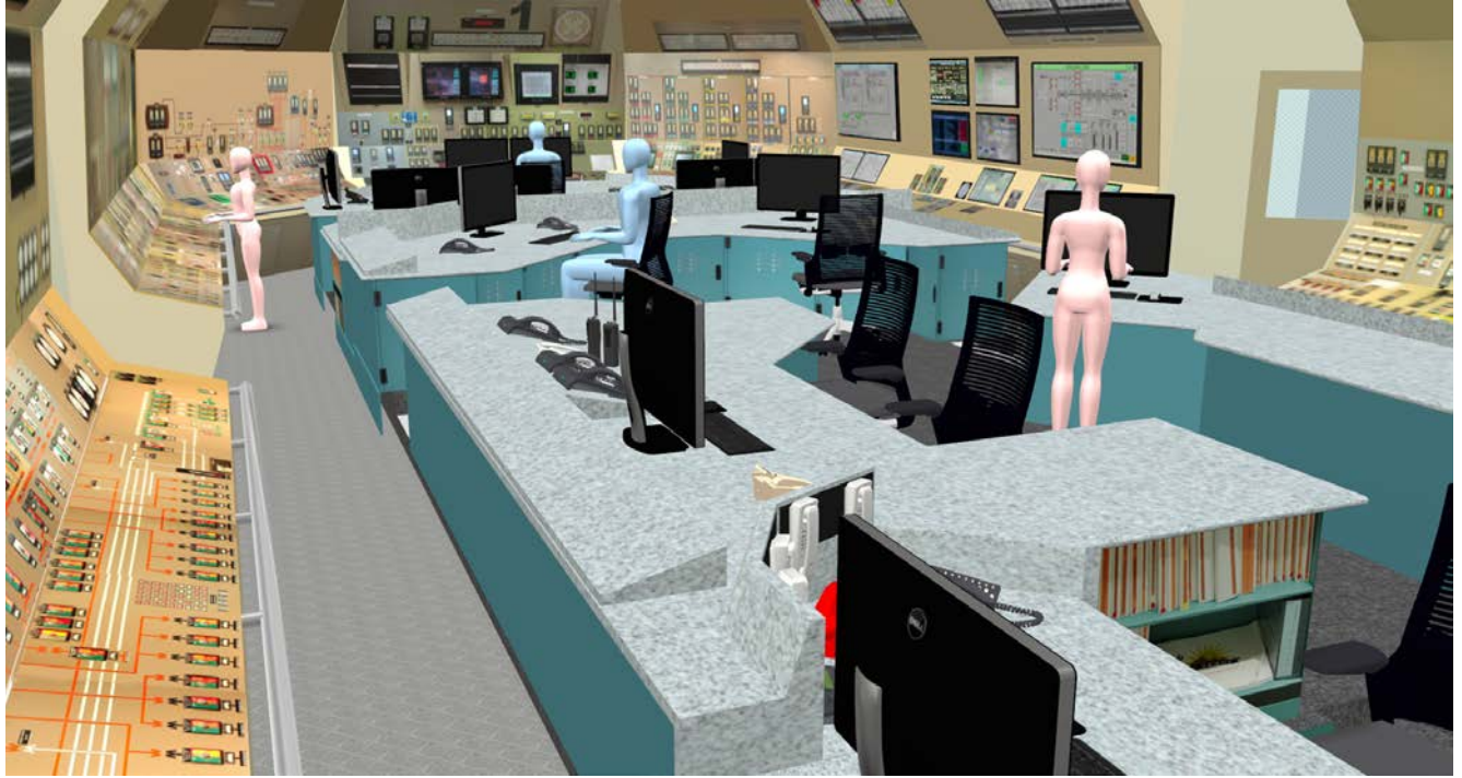
Figure 8 Example of a CREATE drawing of a partial updated Main Control Room (MCR).
