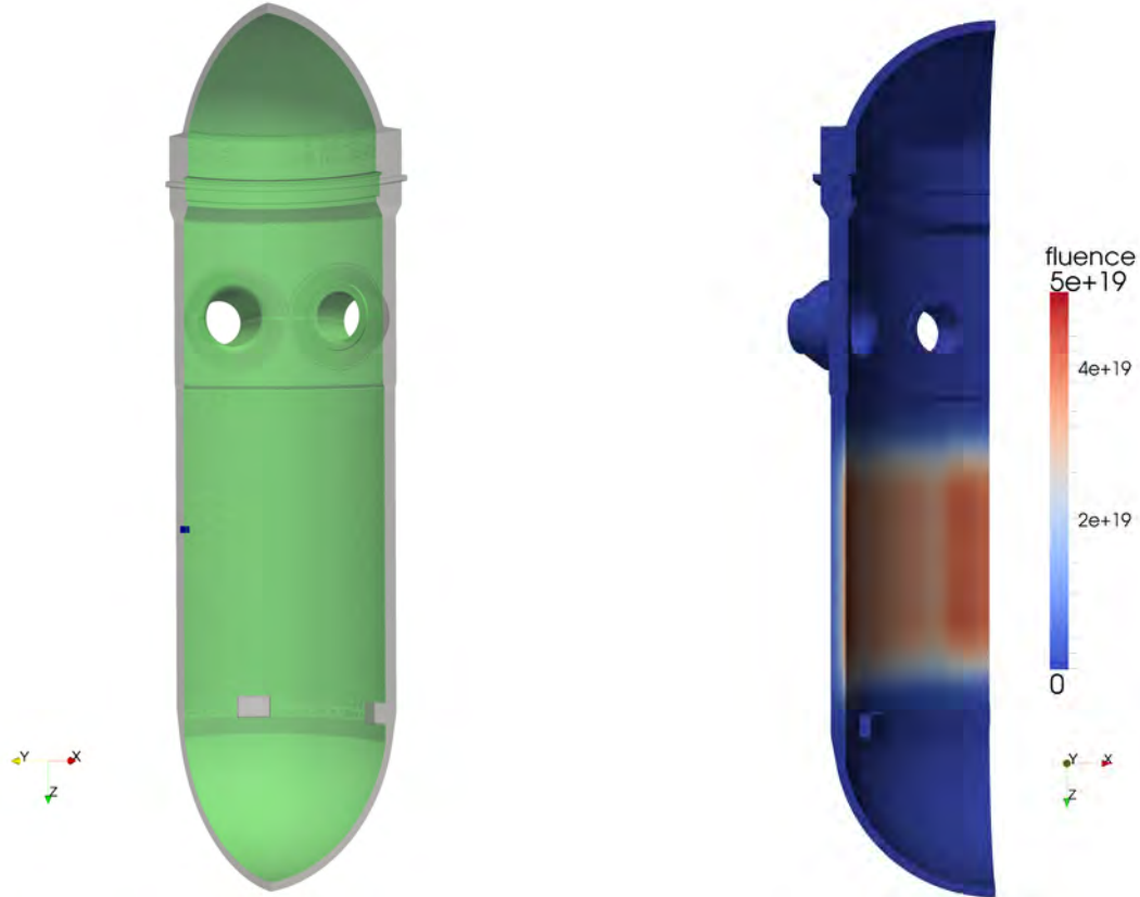
Figure 1: Global model of RPV showing location of submodel with detailed flaw geometry (blue region on left side) (left). The base material is colored gray, and the liner material is colored green. Distribution of accumulated neutron fluence after 32 years of operation (right).
