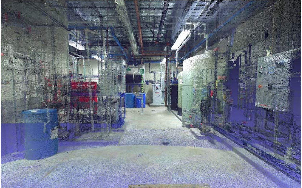
Figure 17. 3D point Cloud Model to Be Converted into a Polygon Mesh and Used in Internal Flooding Simulation.
