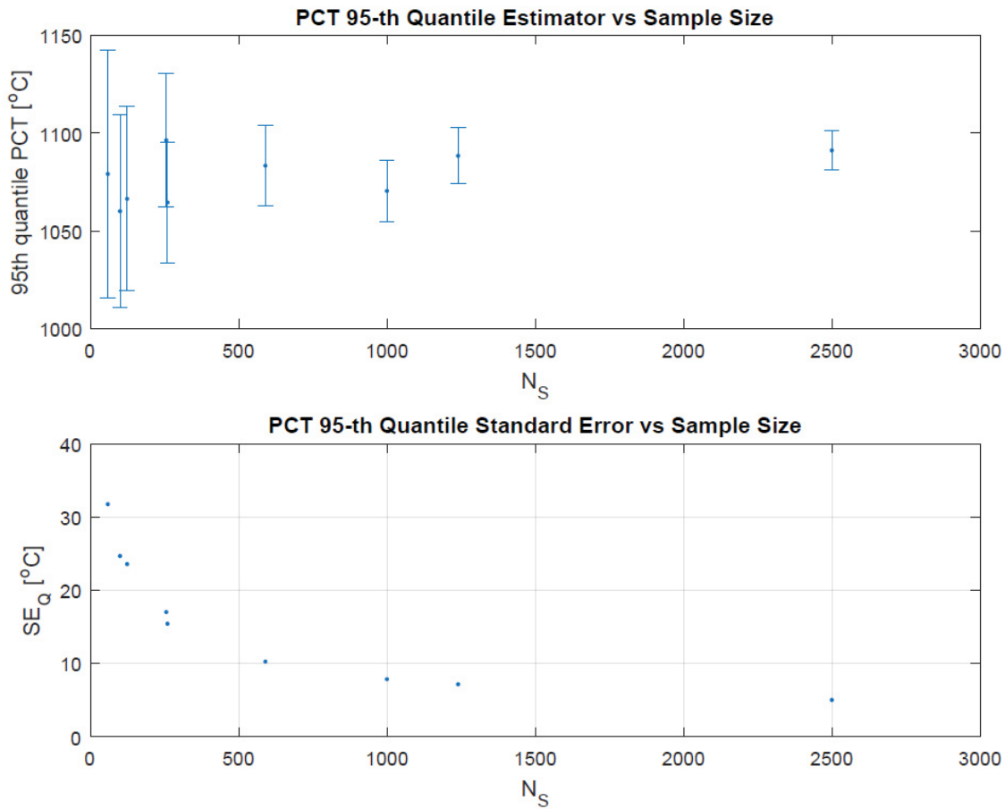
Figure 2-24. PCT 95 th Quantile Estimator 95% Confidence Interval and Standard Error vs Sample Size.
