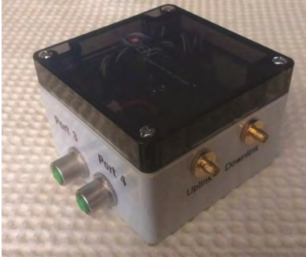
Figure 27. Magnetically attached wireless vibration sensor (EPRI).
