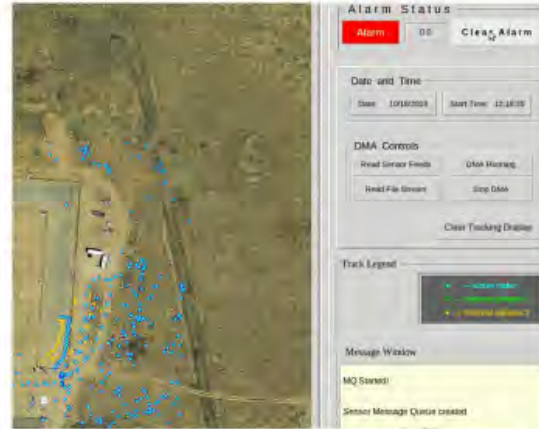
Active Radar (blue) and Thermal Camera (yellow) fused through DMA
