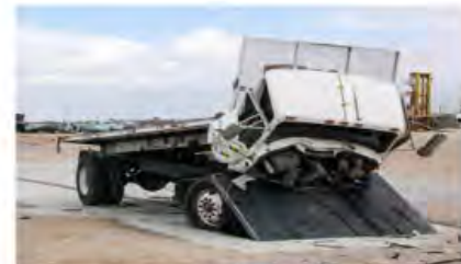
Vehicle Barrier Performance Test
