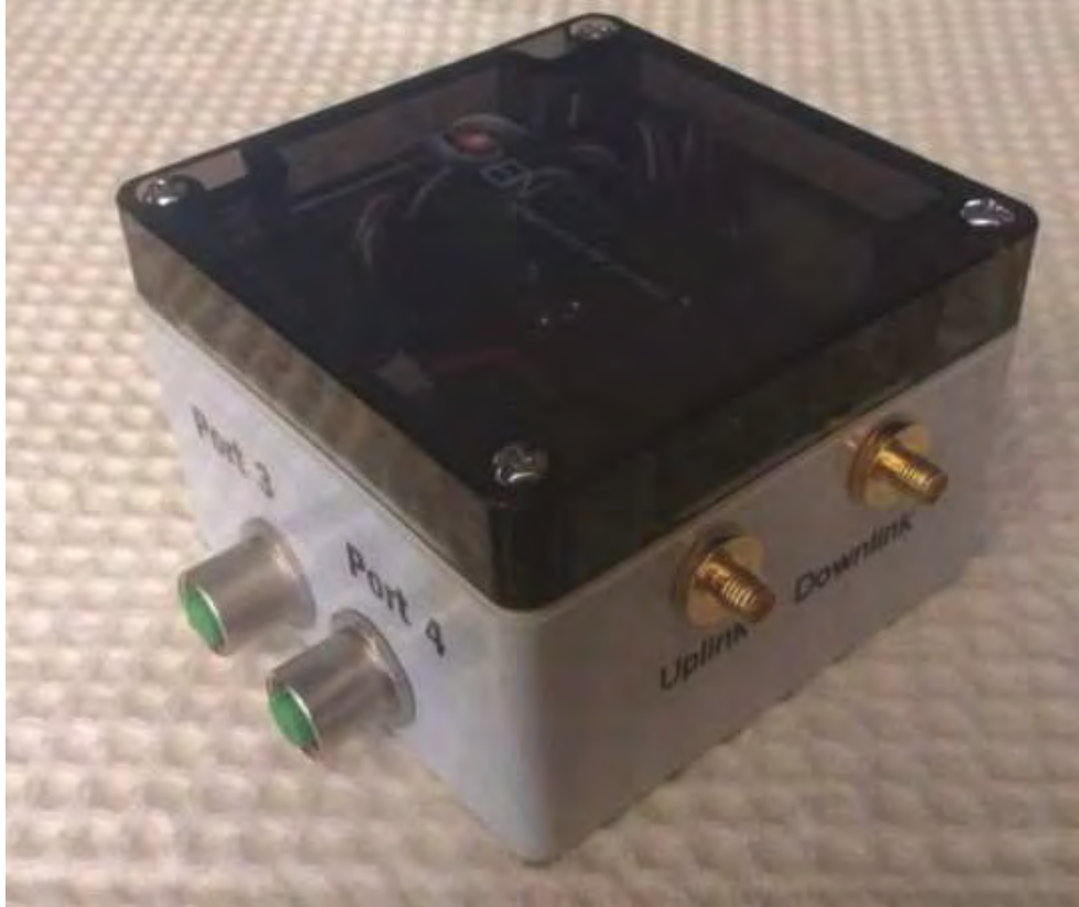
Figure 29. Magnetically attached wireless vibration sensor.
