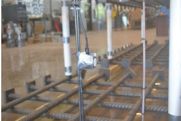
Figure 7.8- An acoustic emission sensor Attached to a positioning bar
