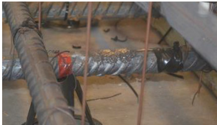
Figure 7.3- Electrical Strain Gauge on the Rebar after Coating
