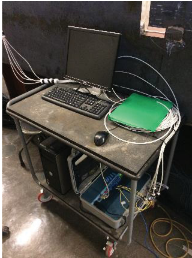
Figure 7.10- SOFO DAQ setup
