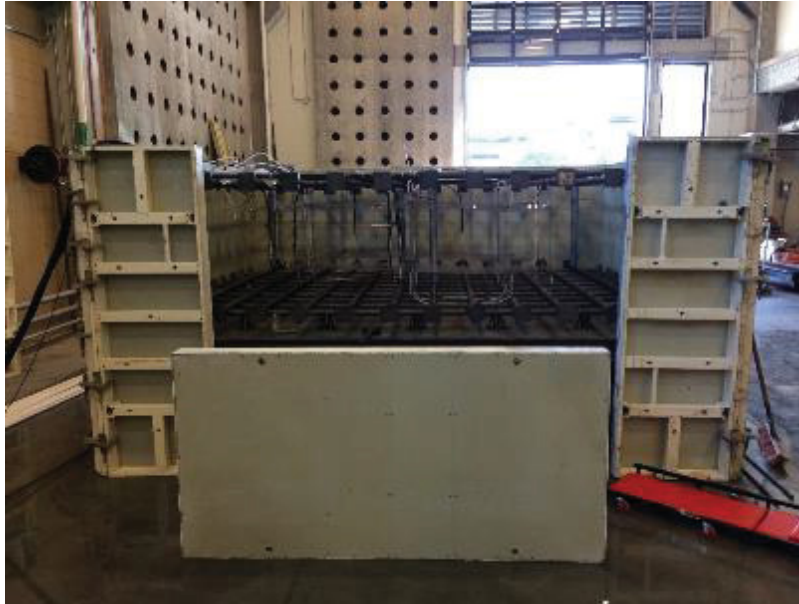
Figure 4.3- Partially assembled side formwork system
