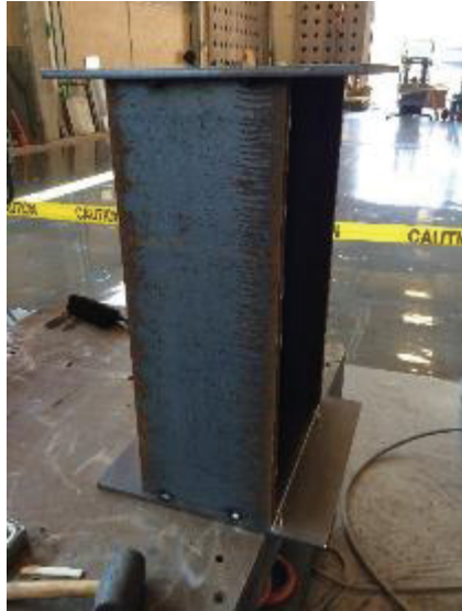
Figure 3.1- Unpainted steel support before welding
