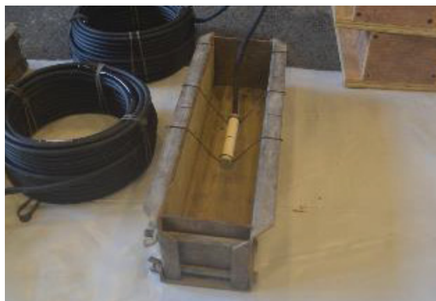
Figure 7.2- Installation of KM strain gages in Creep Specimens
