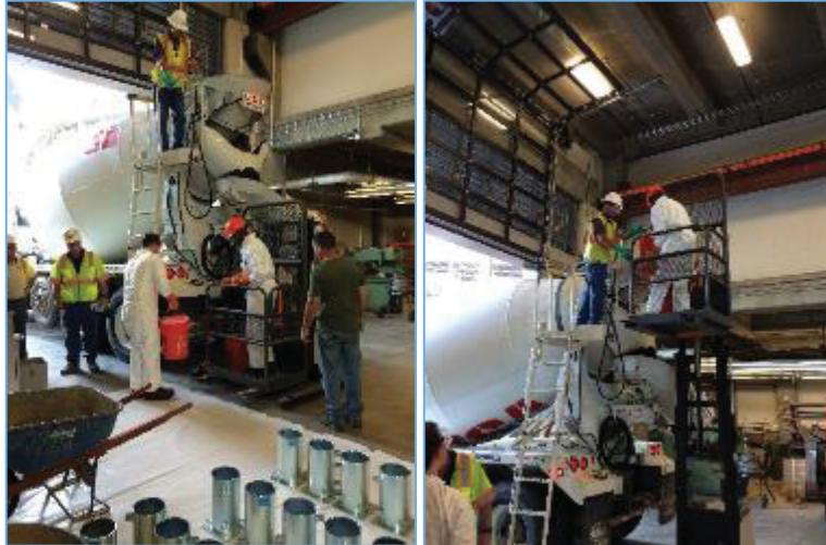
Figure 8.3-. Adding chemicals to a concrete truck
