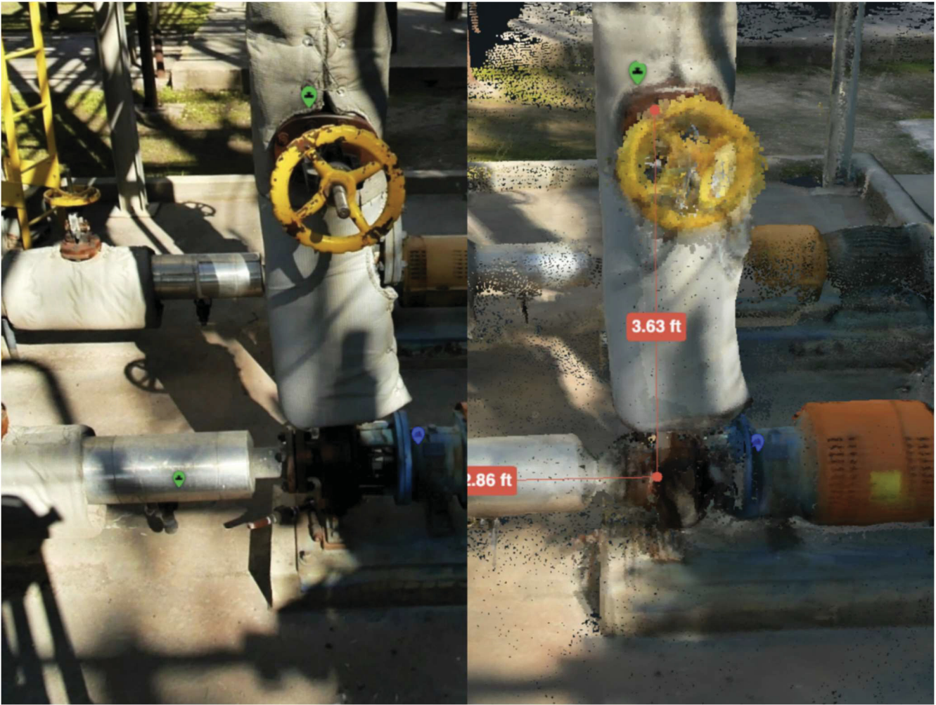
Figure 2. Side-by-side comparison of photogrammetry and LiDAR data collected with mobile mapping and measurement display in the Ei viewer.
