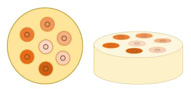
Figure 15. Schematic of epoxy puck containing cable insulation segments for nanoindentation imaging.
