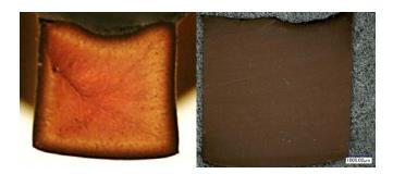
Figure 1. Inhomogeneous aging (Left), possible during rapid laboratory aging (e.g. 180°C for 3 days), can lead to over-prediction of resistance to heat effects compared to homogeneous aging (e.g. 120°C for 60 days) (Right), as would occur in long term service.
