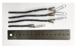
Figure 4. BIW EPR/CSPE (BE15) specimen set
