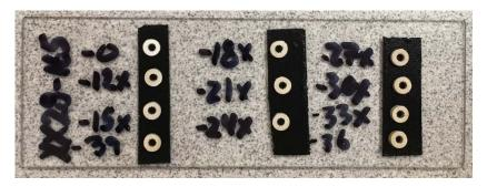
Figure 14. Photo of glass slide containing cross-sections of XX28 XLPE cable aged at 165°C.
