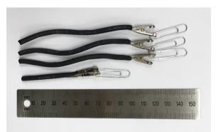
Figure 6. Okonite EPR (OE34) specimen set
