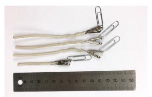
Figure 3. Anaconda EPR (AE21) specimen set
