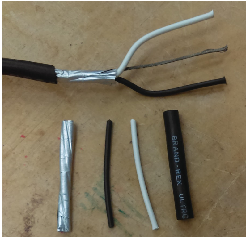
Figure 1. The Brand-Rex Ultrol 600V, shielded #16 gauge instrumentation cable
