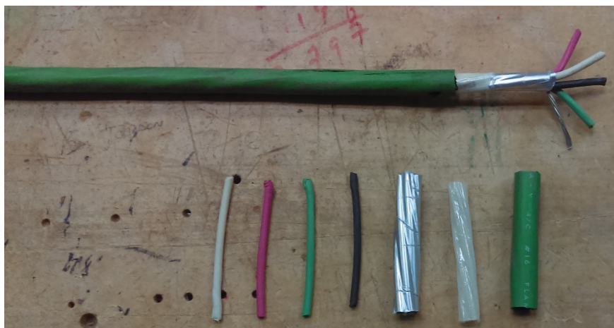
Figure 2. The Anaconda-Y 4/C #16 Flame-Guard FR-EP 600V cable components.
