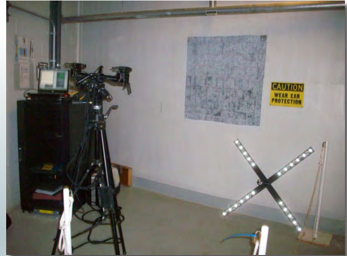
Figure 4. Camera system set up for digital image correlation at the upper containment location.
