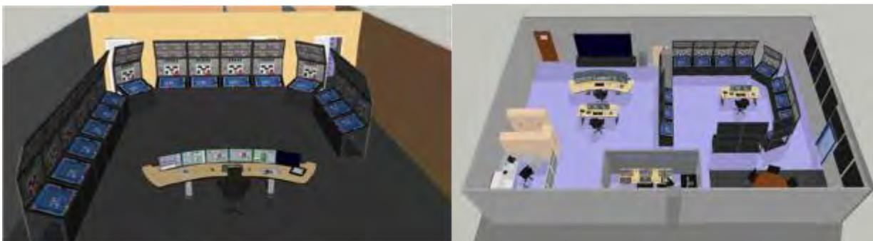
Figure 6. Three-Dimensional Schematic Representations Used in Planning the Layout of the Simulator Buildout.
