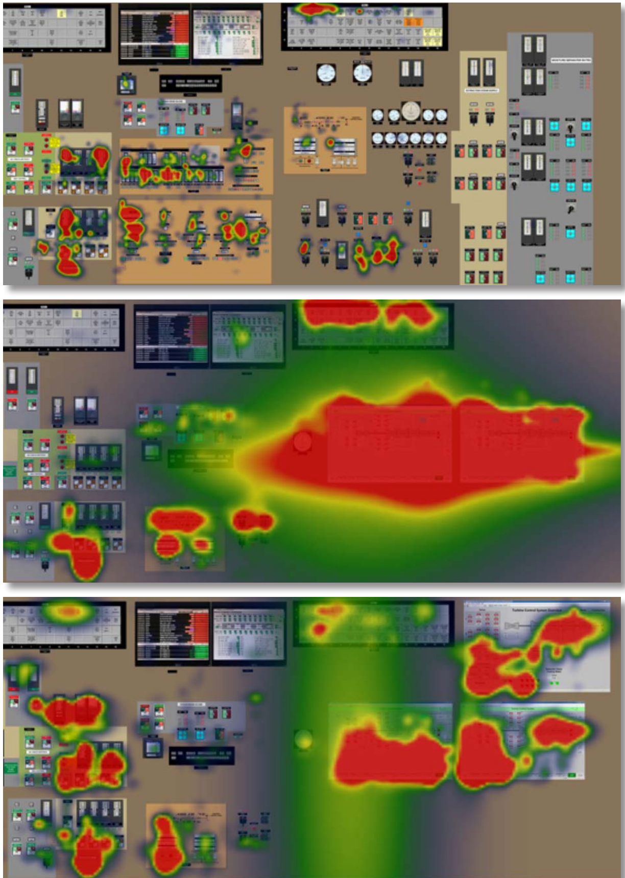
Figure 1: Heat map of eye tracking for analog (top) vs. digital TCS (middle) vs. digital TCS with overview display (bottom).
