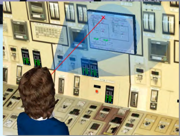
Figure 6. HFE evaluations using three-dimensional modeling to help identify and prevent the introduction of new human error traps when performing digital I&C upgrades (right).
