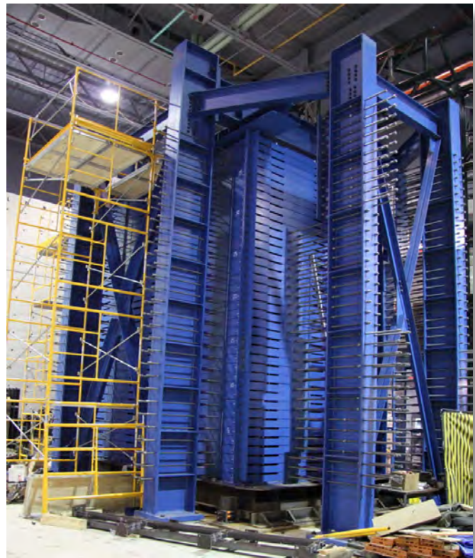
Figure 3. University at Buffalo's geotechnical laminar box.
