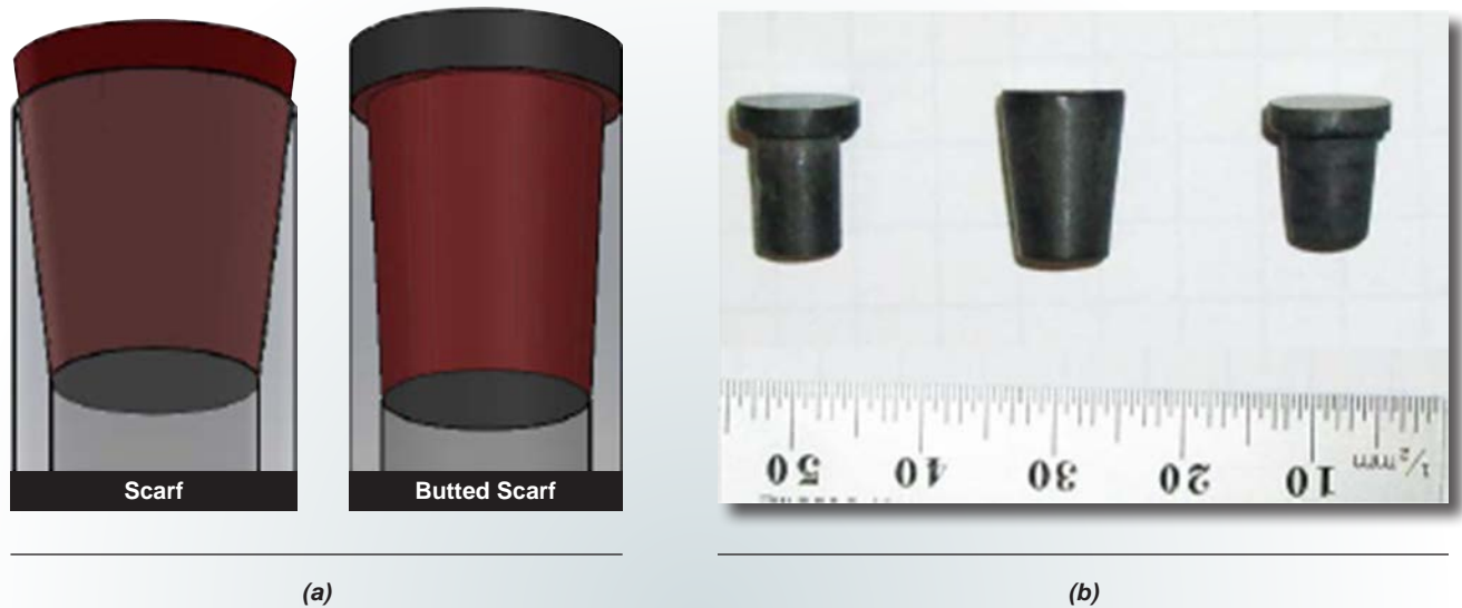
Figure 11. Tested endplug joint geometries for cylindrical joint assemblies: (a) schematic of the scarf and butted scarf geometries inserted into the cylindrical cladding tube, and (b) as-fabricated monolithic silicon carbide butted scarf (left), scarf (middle), and butted lap endplugs.
