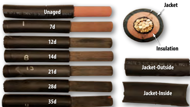
Figure 7. Pink EPR insulation; chlorinated polyethylene jacket aged samples with jacket removed from half of the sample.
