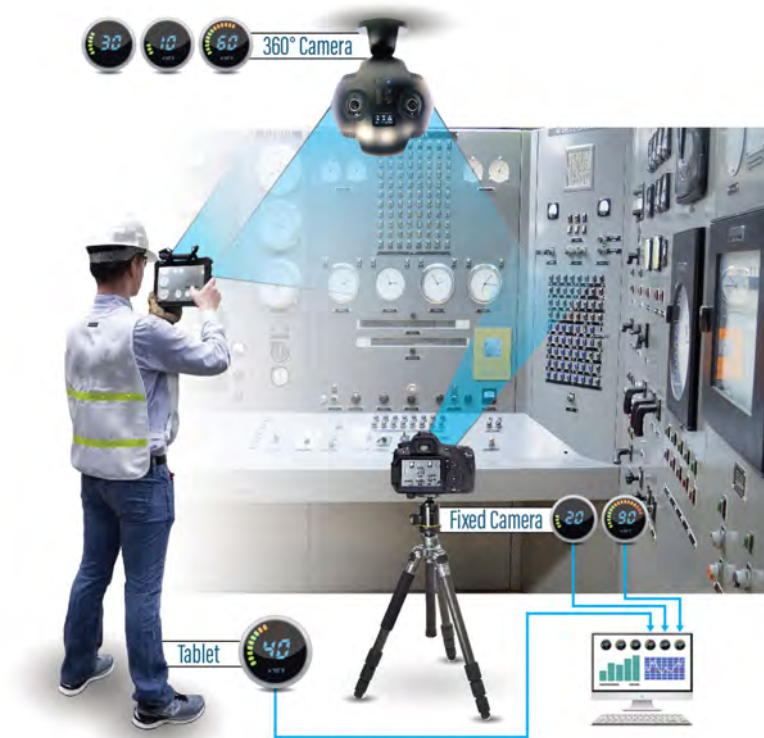
Figure 8. Uses of automated gauge reading at oblique angles.
