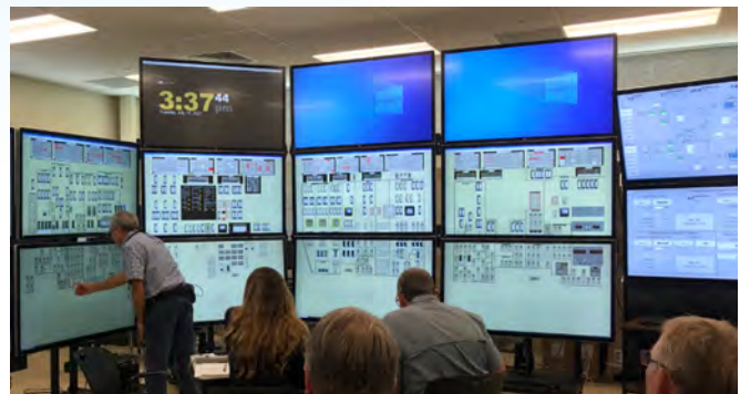
Figure 2. Operators performing scenarios to evaluate the impact of thermal dispatch on existing operations to evaluate the existing system design and human-system interface.
