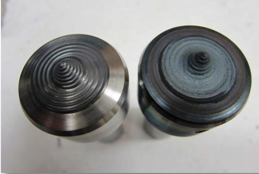
**Figure 14. Polycrystalline cubic boron nitride tools: new condition (left) and after welding (right).**
