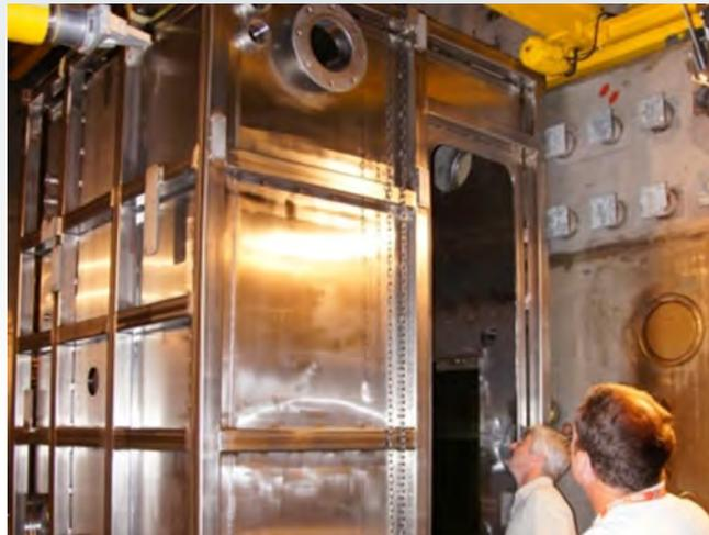
**Figure 12. Welding cubicle undergoing a preliminary fit test in the hot cell.**
