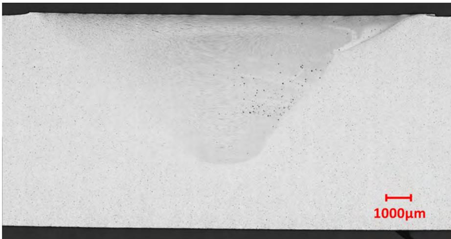
**Figure 17. Cross-section of a friction stir weld on He-containing 304L.**
