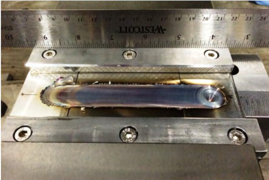
**Figure 15. FSW on 304L specimen (weld path is from left to right).**
