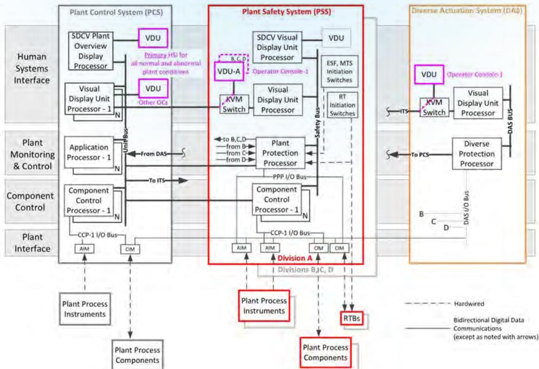
– electrical, physical, communication and functional. High availability and prevention of erroneous control actions are achieved without adding redundancy that is not needed for single failure criterion compliance. The diverse actuation system is a novel design with no input/output modules of its own, providing a cost-effective means to cope with digital common cause failure in the plant safety system.
