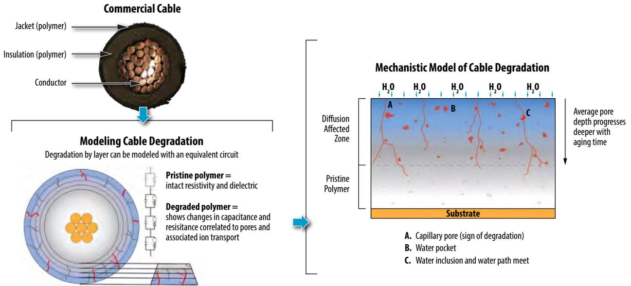
Figure 6. Mechanistic model to describe the degradation of the cables by water intrusion.
