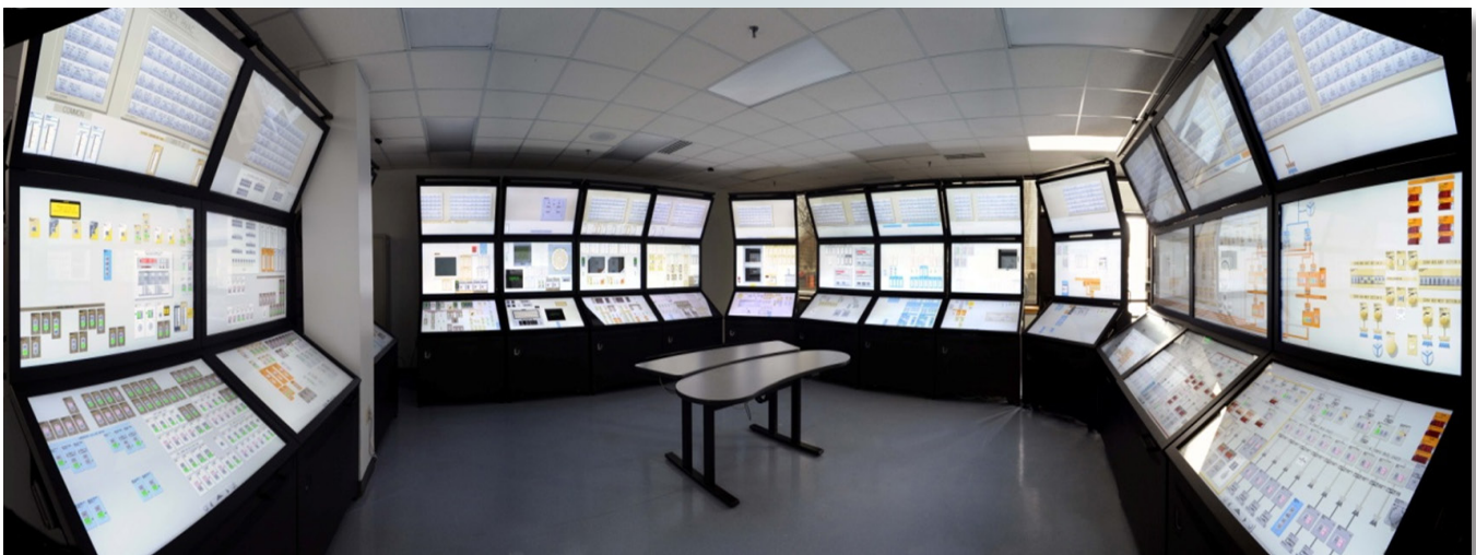
Figure 11. HSSL configured with bench-board-style control bays for realistic simulation of current LWR control rooms.
