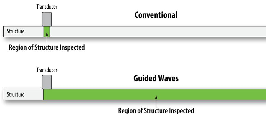
Figure 12. Inspection of UGWs versus conventional UT inspection [3].
