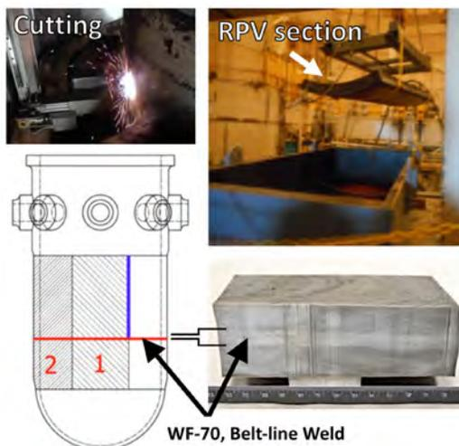
**Figure 9. Sectioned blocks from the RPV segment with block IDs and RPV orientation markings: The Y axis is perpendicular to the beltline weld; the X axis is parallel to the beltline weld with arrow pointing away from the high-fluence edge.**
