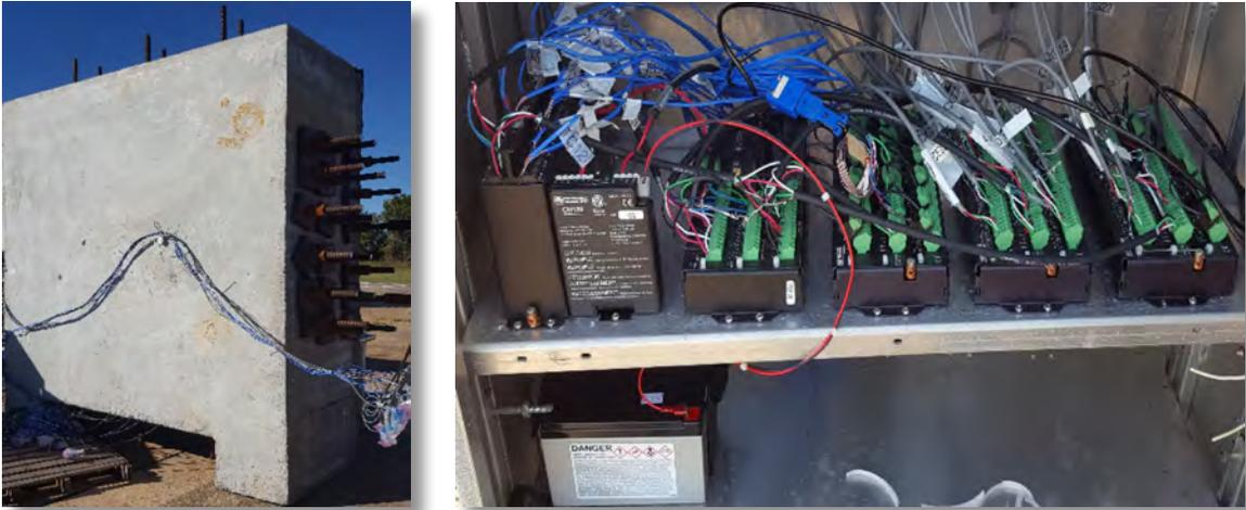
**Figure 7. Validation of the structural model is being achieved via large-scale mock containment structure wall sections. The walls are exposed to loads similar to that in real structures and heavily instrumented with concrete and steel strain gages (to detect creep effects), temperature sensors, and humidity sensors. Grizzly model predictions will be compared to measured values.**
