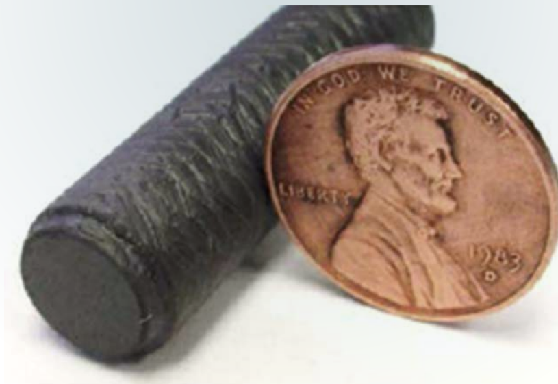
Figure 3. Silicon carbide–silicon carbide composite assembly (General Atomics).
