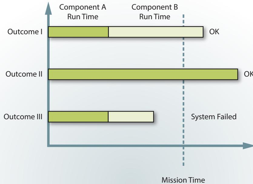
**Figure 2. Failure or success time concept for two components in a switch-type system**
