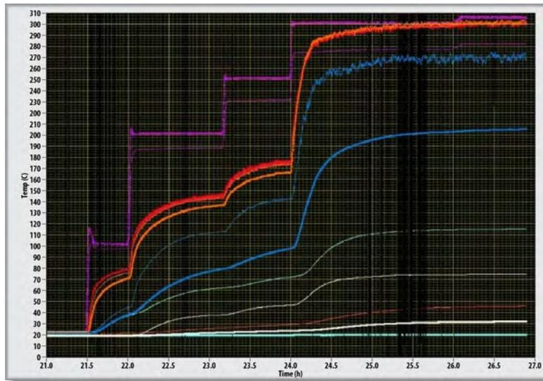
Figure 6. Data acquisition system screen shot showing various thermocouple readings during the heat-up session of a PWR environment fatigue test.
