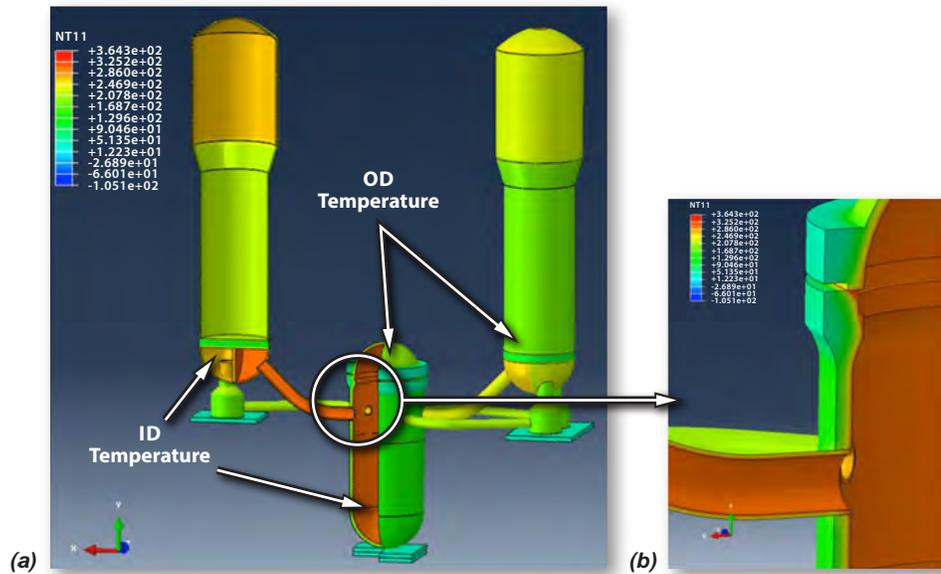
**Figure 8. Results from 3-D heat transfer analysis for the PWR model during the peak of a reactor thermal cycle: (a) inner diameter (or ID) and outer diameter (or OD) surface temperature (in degrees Celsius) distribution of different components, and (b) example temperature gradient across the reactor pressure vessel shell thickness.**
