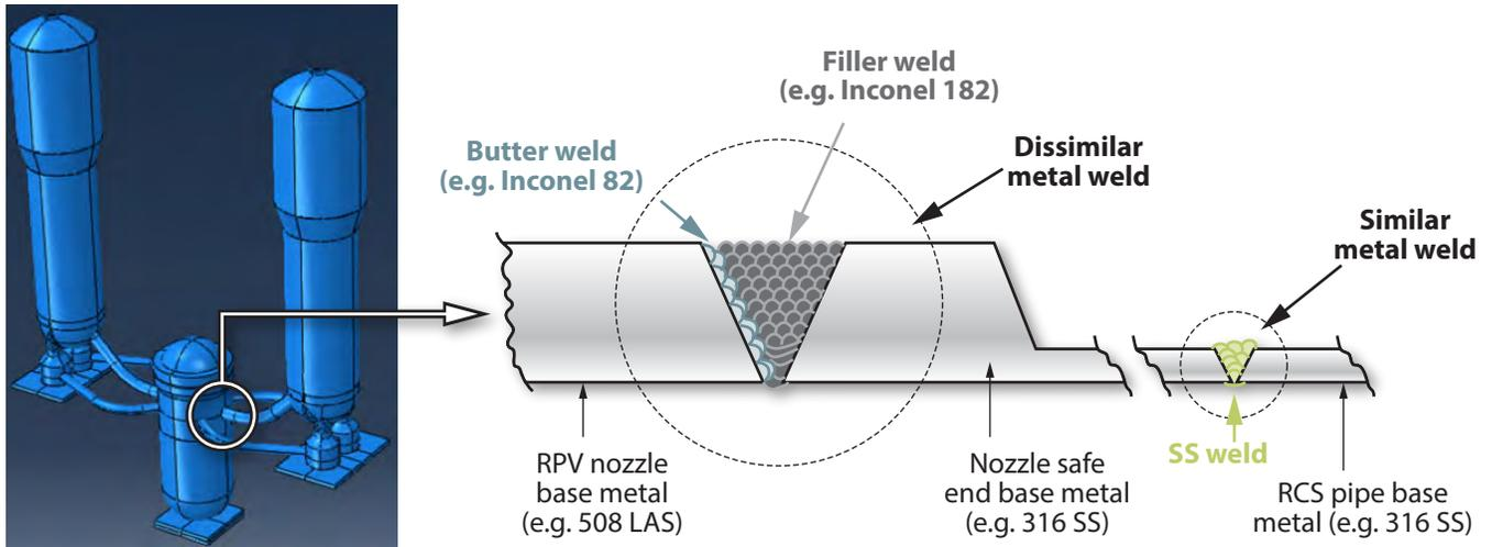
**Figure 4. Computer modeling schematic of a PWR showing different metals and welds used in the reactor pressure vessel, RCS pipe, and their joints.**
