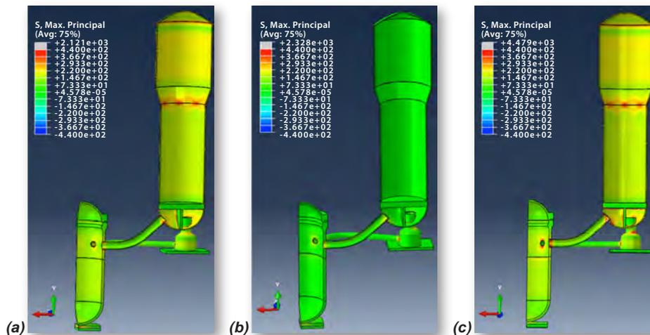
Figure 9. Results from a 3-D thermal-mechanical stress analysis showing the maximum principal stress (in MPa) distribution in a PWR during peak (a) pressure loading, (b) thermal loading, and (c) both pressure and thermal loading.
