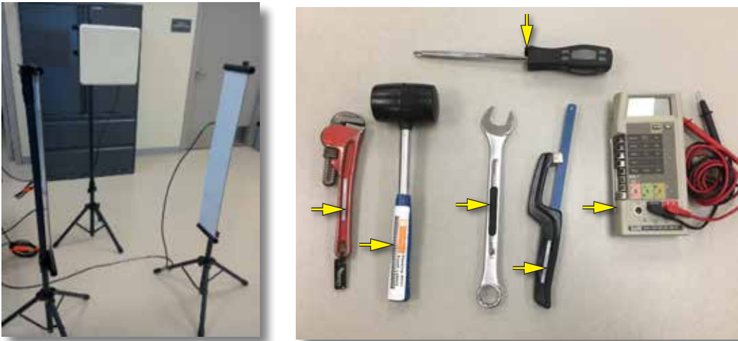
Figure 20. Radio frequency identification of tools for foreign material exclusion.
