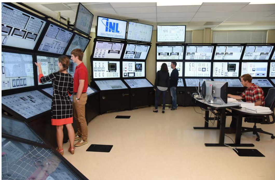
Figure 13. Human Systems Simulation Laboratory, a full-scale, full-scope simulation facility.
