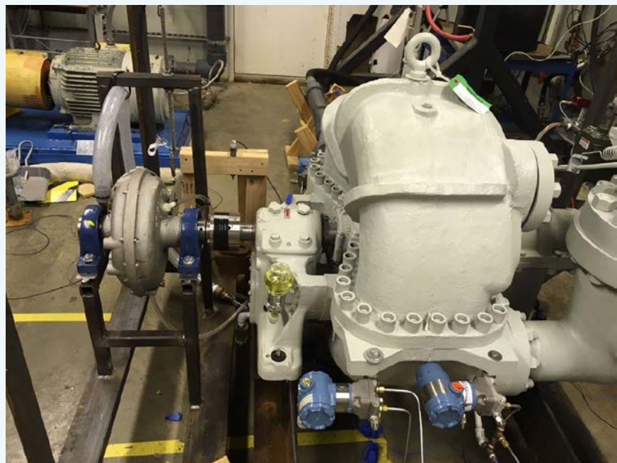
Figure 13. Crystal River-3 Terry Turbine (GS-2) used for testing.
