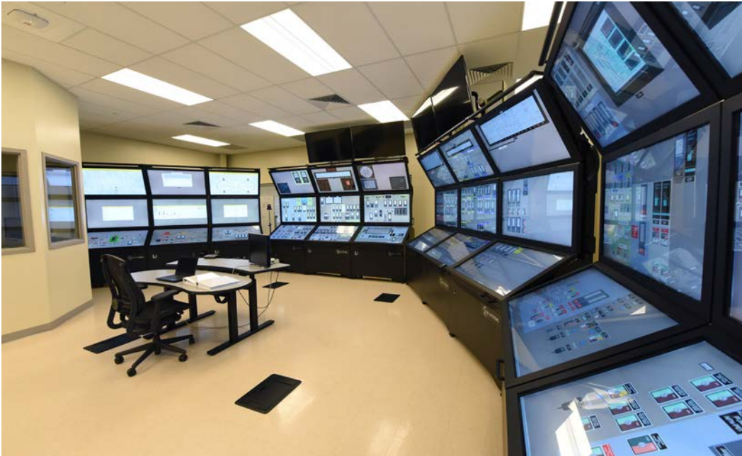
Figure 29. Human Systems Simulation Laboratory: a reconfigurable hybrid control room simulator.
