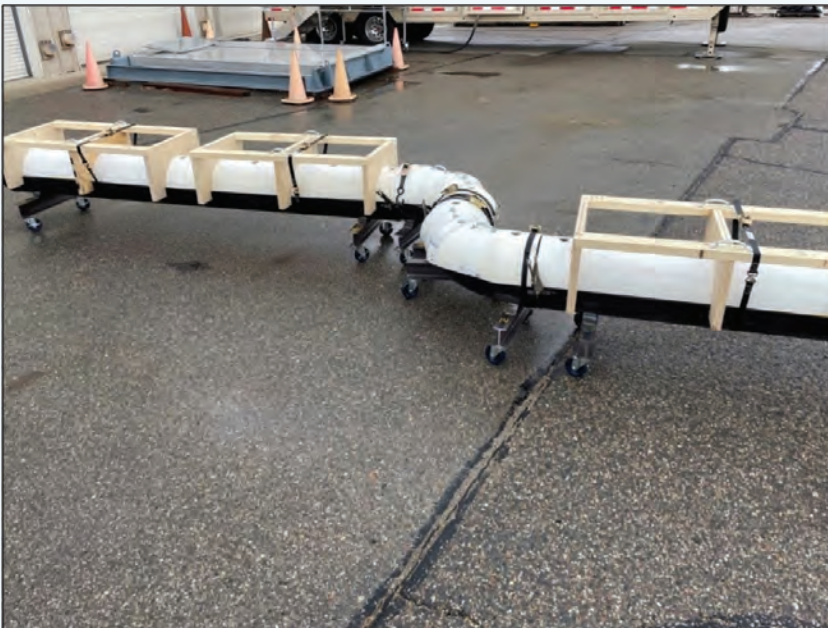
Figure 24. Three-Dimensional Piping Structure in an S-shape Configuration.
