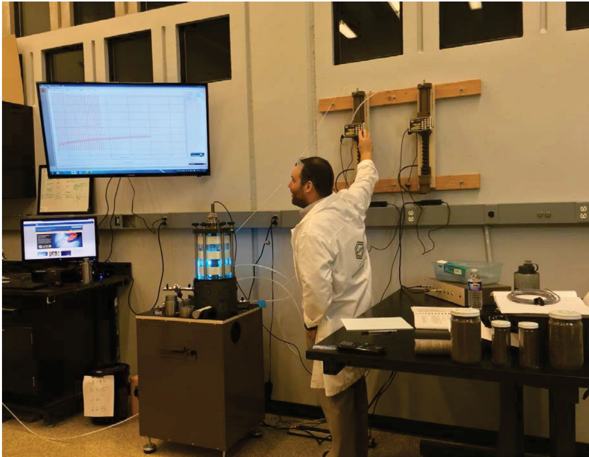
Figure 7: Cyclic Triaxial Machine at University at Buffalo
