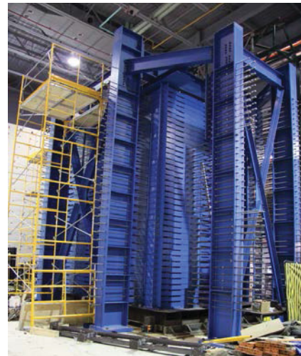
Figure 1: University at Buffalo geotechnical laminar box
