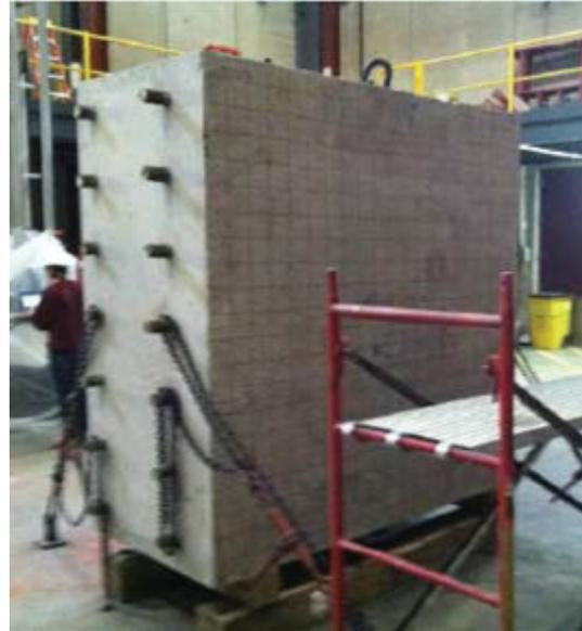
**Figure 3. Rough surface of the specimen [1].**
