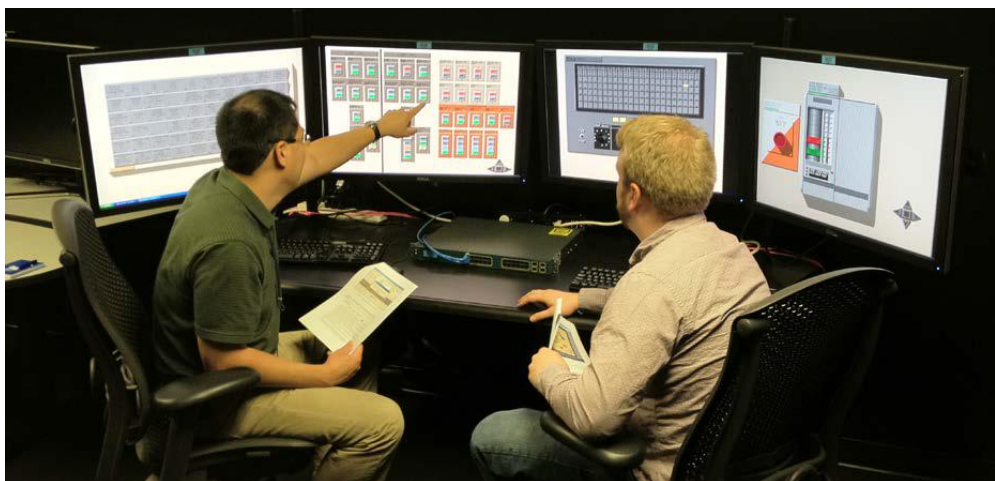
Figure 13 Human Systems Simulation Laboratory used to evaluate advanced control room technologies
