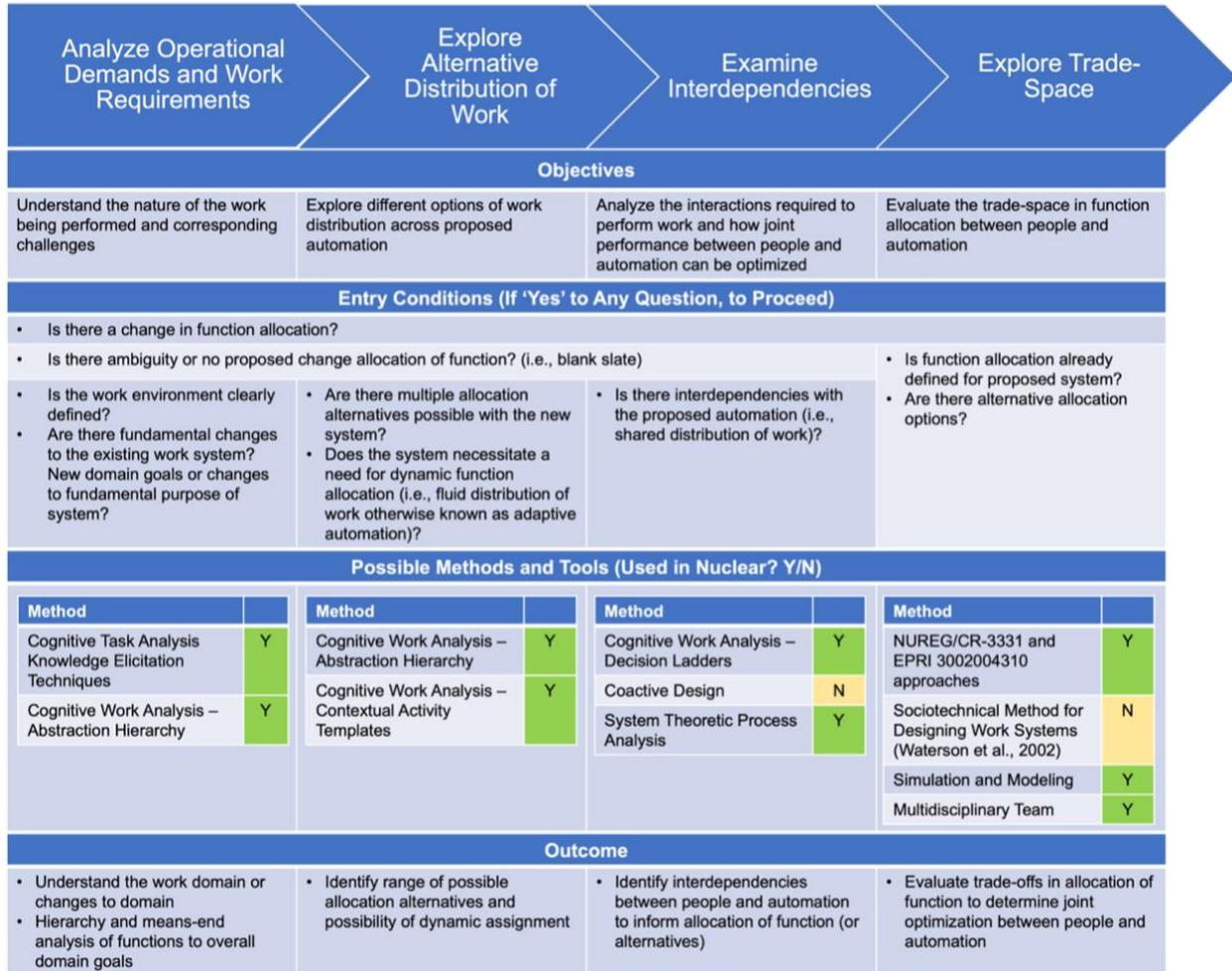
Figure 40. Integrated function allocation toolset (adapted from INL/RPT-22-68472).
