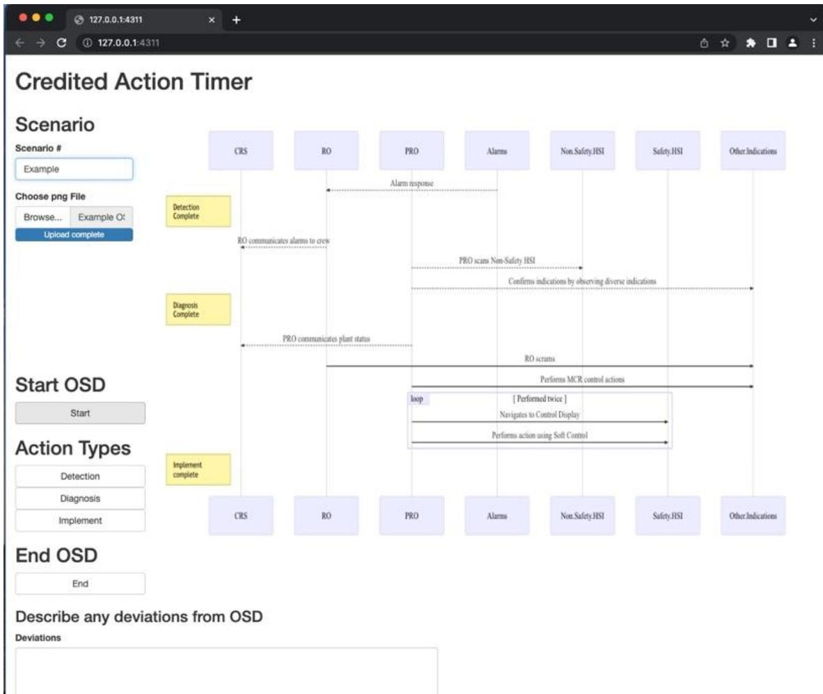
Figure 26. Custom timeline analysis tool with generic OSD presented (adapted and enhanced from INL/RPT-23-71395).
