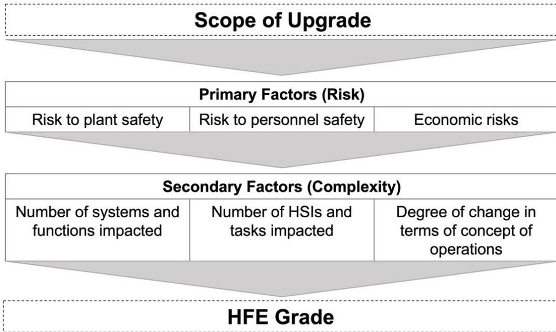
Figure 14. HFE grading considerations (adapted from INL/RPT-22-70538).
