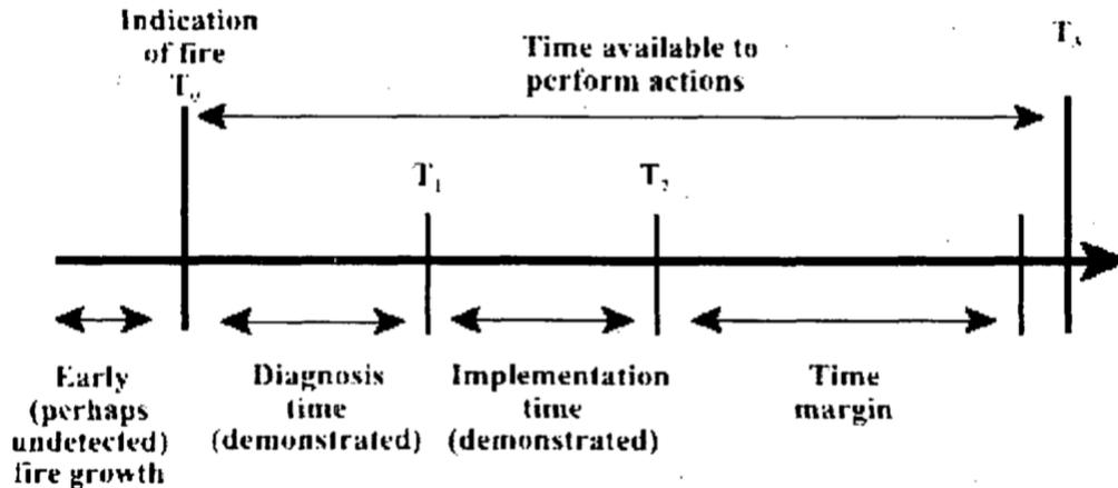
Figure 23. Timeline guidance for evaluating manual operator actions (adapted from NUREG-1852 2007).
