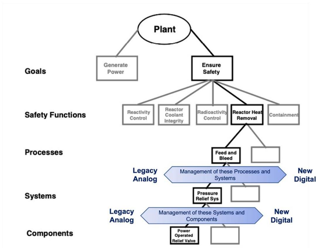
Figure 37. Vertical slide through a plant's functional hierarchy for ensuring safety (adapted and enhanced from NUREG-0711 2012).
