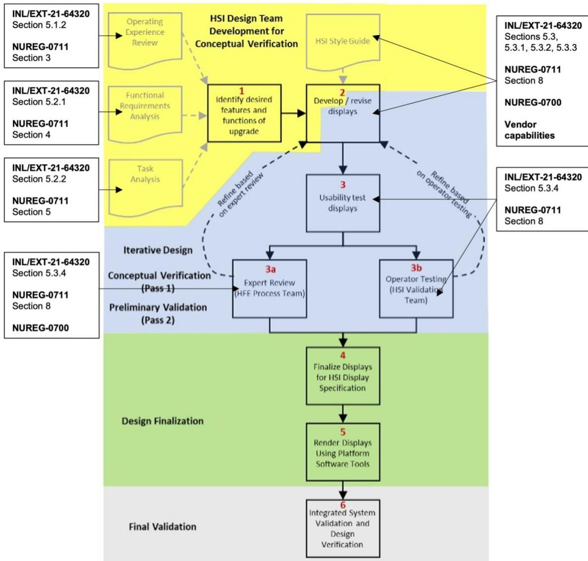
Figure 20. Iterative process used for preliminary validation (adapted and enhanced from INL/RPT-23-71395).
