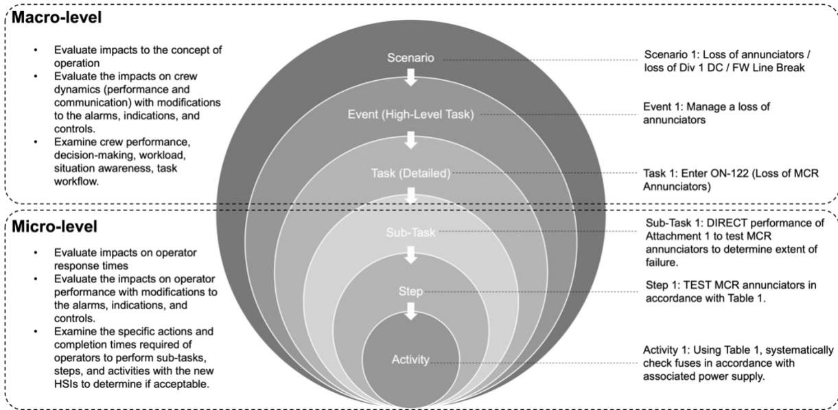
Figure 16. Decomposition of tasks for performing task analysis (adapted from INL/RPT-22-68472).
