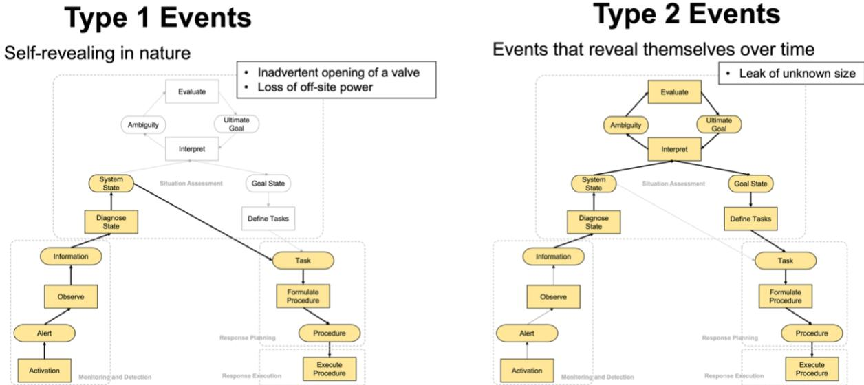
Figure 24. Types of manual actions as characterized by decision ladders from cognitive work analysis (adapted from INL/RPT-23-71395).
