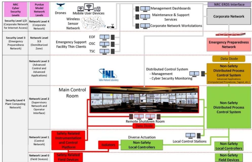
Figure 6. Simplified digital infrastructure (adapted from INL/EXT-21-64580).
