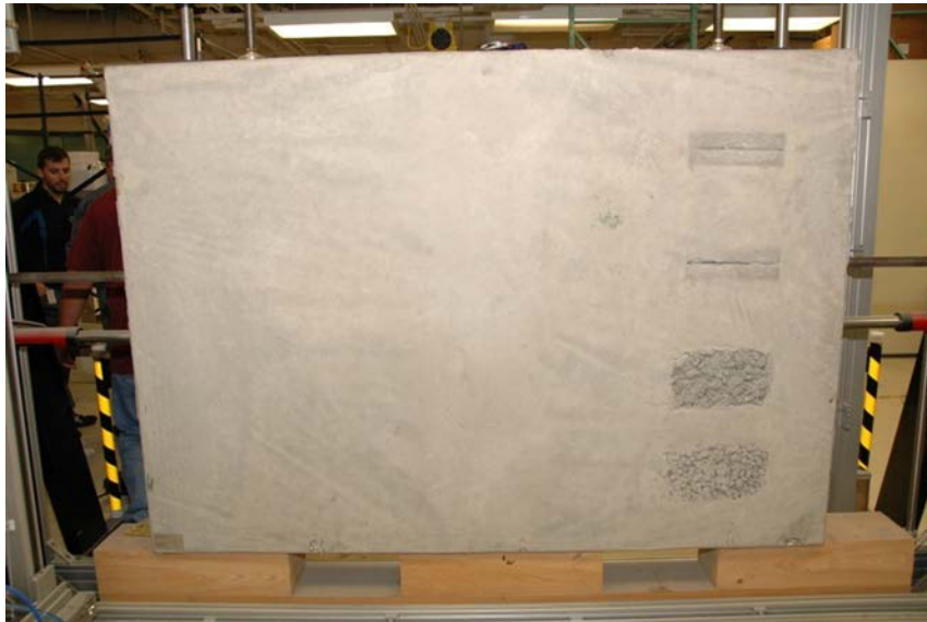
Figure 6. A concrete test specimen from the Florida Department of Transportation's State Materials Office NDE Validation Facility in Gainesville, FL with simulated cracking and non-consolidation flaws (Clayton, 2014).
