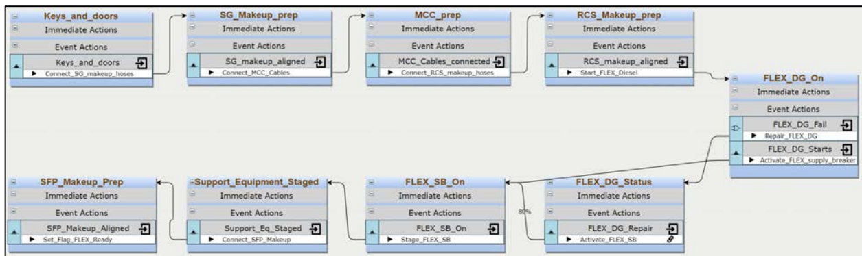
Figure 14. Sequential preparation of FLEX equipment.
