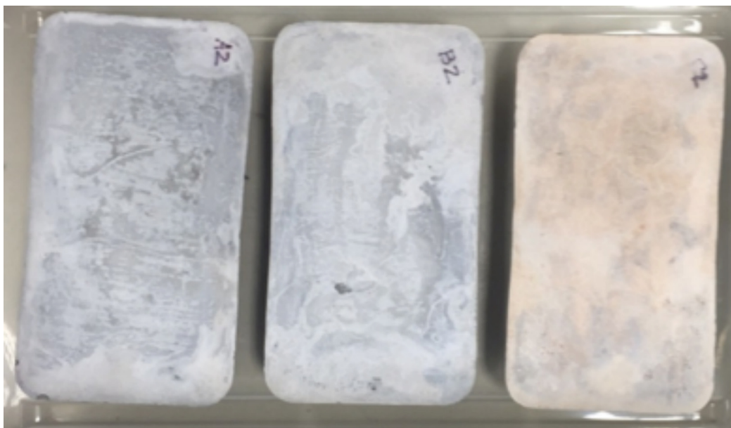
Figure 21. Samples after 14 days of curing in NaOH solution.
