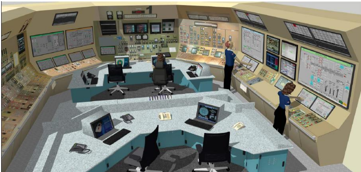
Figure 6. Concept Design for an Advanced Hybrid Control Room
