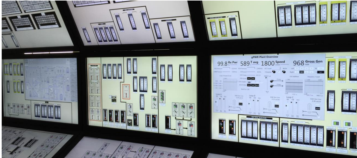
Figure 8. Computerized Operator Support System Depicted in a Control Board
