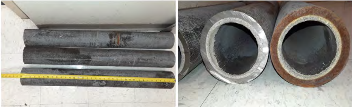
Figure 36. Ductile iron pipe samples.
