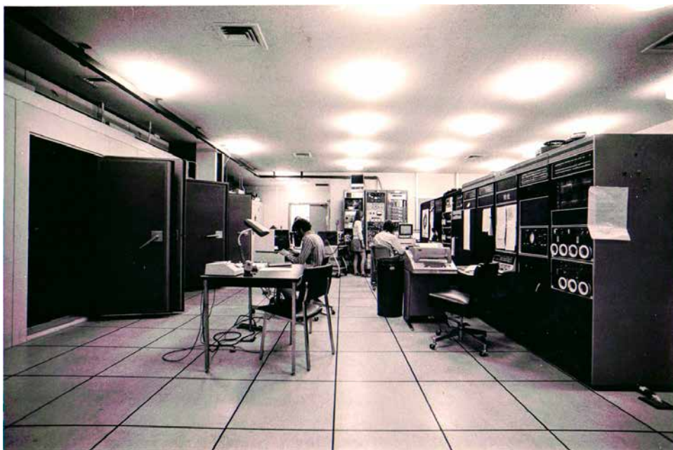
Two computers—a Digital Equipment Corporation PDP-9 and a PDP-15—in the UC San Diego Psych Lab of Peter Lindsay, Don Norman, and Dave Rumelhart in the early 1970s. Graduate students are shown working with acoustically isolated chambers on the left where the experiments could be done free of distraction from the noise of the lab.
