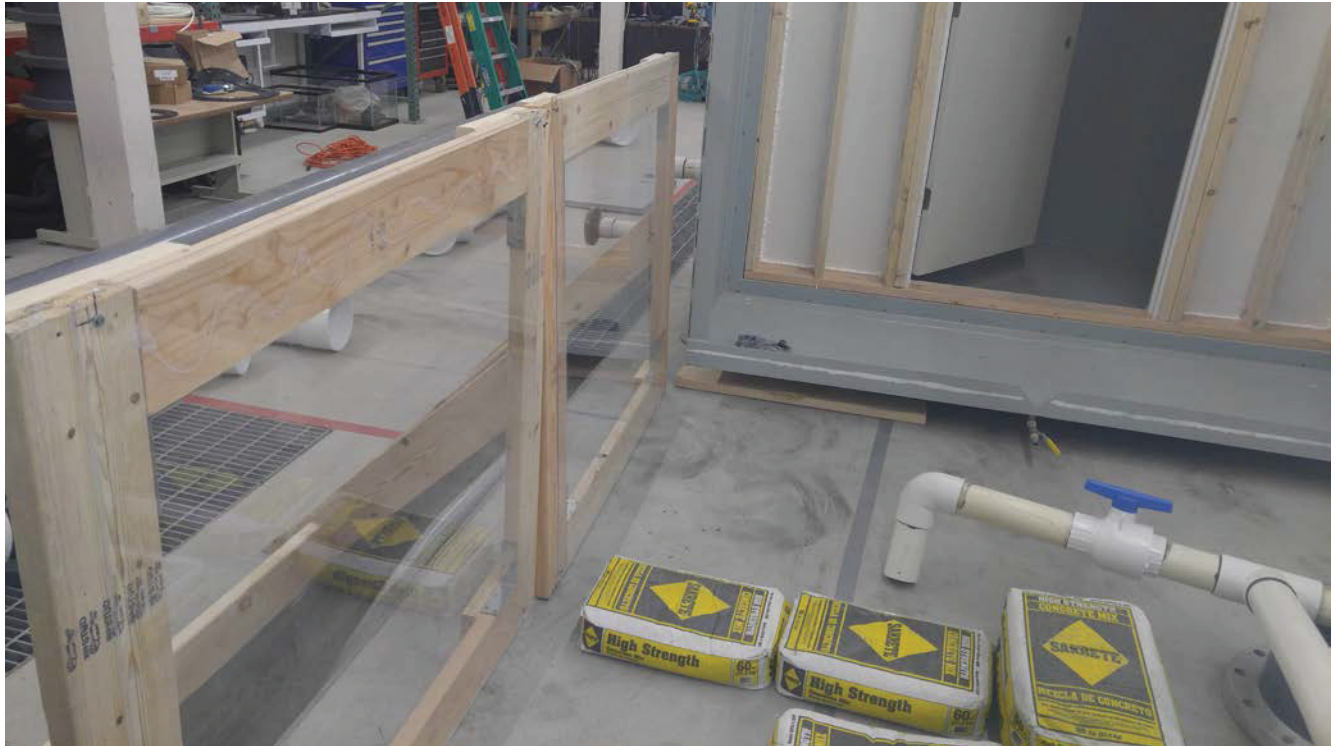
Figure 9. Acrylic sheeting splash guard.
