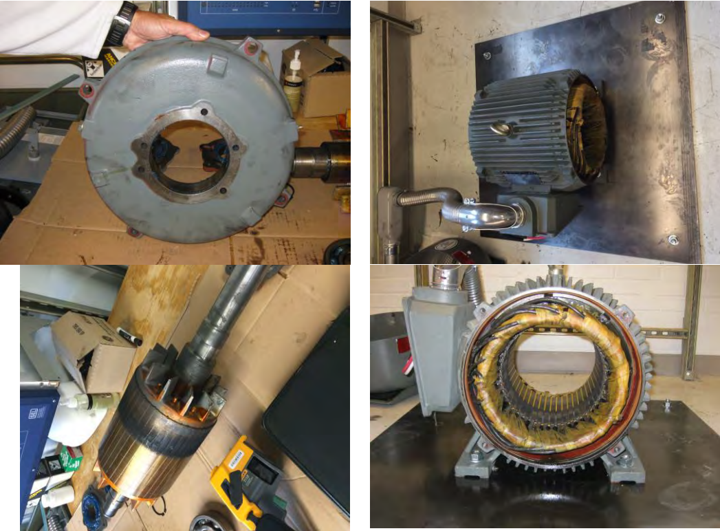
Figure 20. Selected portions of disassembled motor after loss of bearing lubrication and presence of contaminant test.
