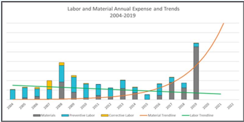
Figure 24. Sample system labor and material cost analysis.
