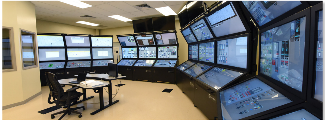
Figure 23. Human Systems Simulation Laboratory: a reconfigurable hybrid control room simulator.
