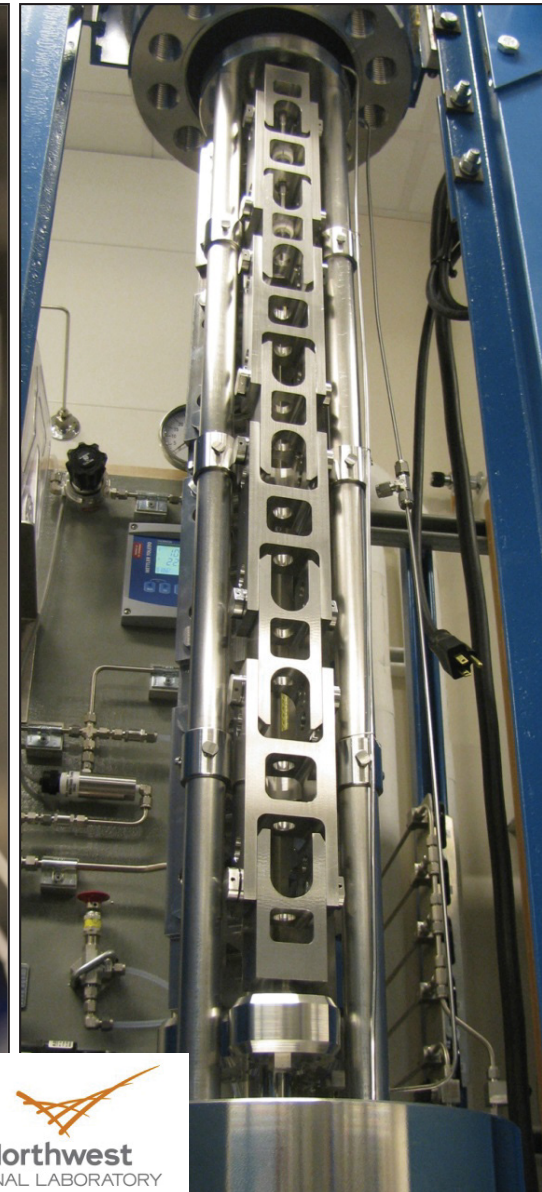
36-Specimen SCC Initiation System
