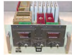
Digital meters upgrade - Factory installed during a new drawer build
