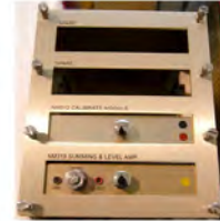
Improved card cage with captive screws
