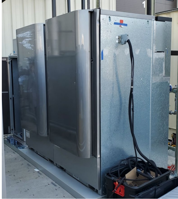
Figure 9. Photograph of the Bloom prototype 100 kW HTE system under testing at INL.
